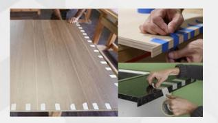
Apply masking tap on the edges & keep under pressure. Handling strength is received with in 1-2 hours, so finishing work can start. Full strength will be achieved with in 24 hours under room temperature.
