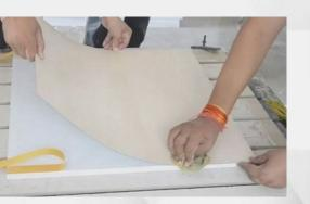
Once the tack is formed and the film turns transparent, paste the both the substrates properly. Bring both the PVC / Acrylic sheet substrates coated with **HAMMER SHIELD** in contact and make proper alignment.
