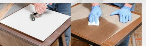
Press the laminated portion by using wet squeezed cloth to remove air entraption.
