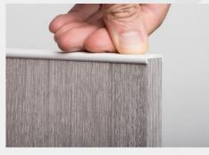
Join PVC Edge Banding & apply pressure uniformly to ensure excess glue oozing out from the joint portion. Remove softly and carefully using cloth / cotton.
